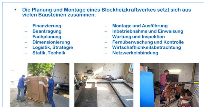
Figure 15. Planning and installation of a combined heat and power generation plant (The planning and installation of a combined heat and power generation plant has many components: financing, application, specialist planning, dimensioning, logistics, strategy, statics, technology, installation and implementation, commissioning and training, maintenance and inspection, remote monitoring and control, profitability analysis, network integration)
